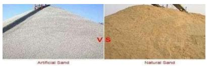
Artificial sand, also called crushed sand or mechanical sand, refers to rocks, mine tailings or industrial waste granules with a particle size of less than 4.75 mm, which are processed by mechanical crushing and sieving, but does not include soft and weathered granules.
