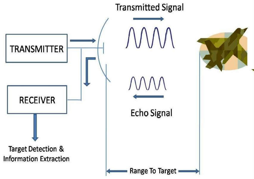
[ BLOCK DIAGRAM OF A SIMPLE RADAR SYSTEM ]
