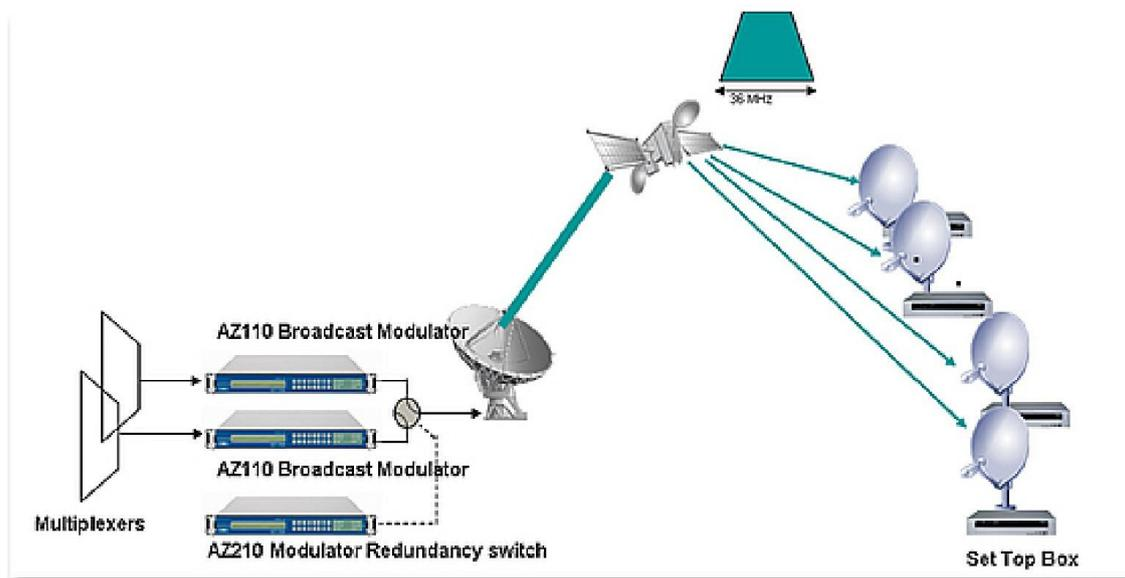
The receive antenna may be permanently pointed at the satellite, which is at a fixed point in the sky, in a geostationary orbit.
