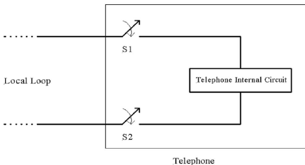
When a handset is picked up, a DC current ranging between 20 and 120 mA flows on the pair of wires connecting the telephone to the CO. This current flow causes a relay coil to magnetize and its contacts close.
