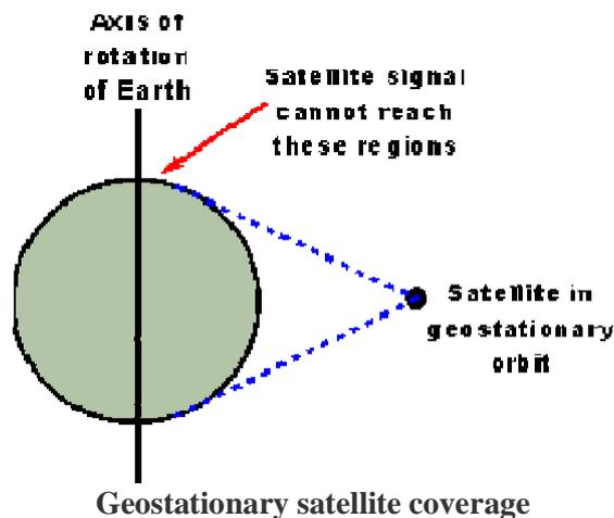
For a constellation of three satellites equally spaced around the globe, it is possible to provide complete coverage around the equator and up to latitudes of 81° both north and south.
