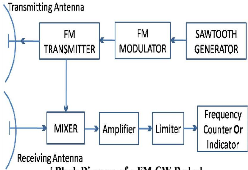
[ Block Diagram of a FM-CW Radar ]
