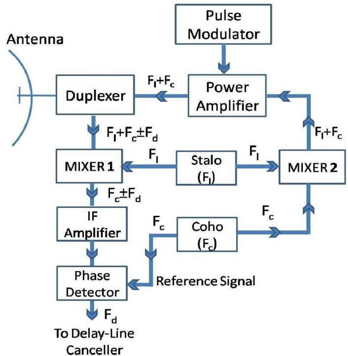
[ BLOCK DIAGRAM OF A **MTI RADAR SYSTEM** ]
