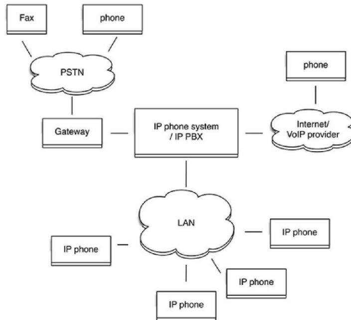
At the same time you are gaining many technical advantages by using IP technology for your telephony. Users of an VoIP phone system simply plug their IP phone into the nearest LAN port. Then, the IP phone registers automatically at the VoIP phone system.
