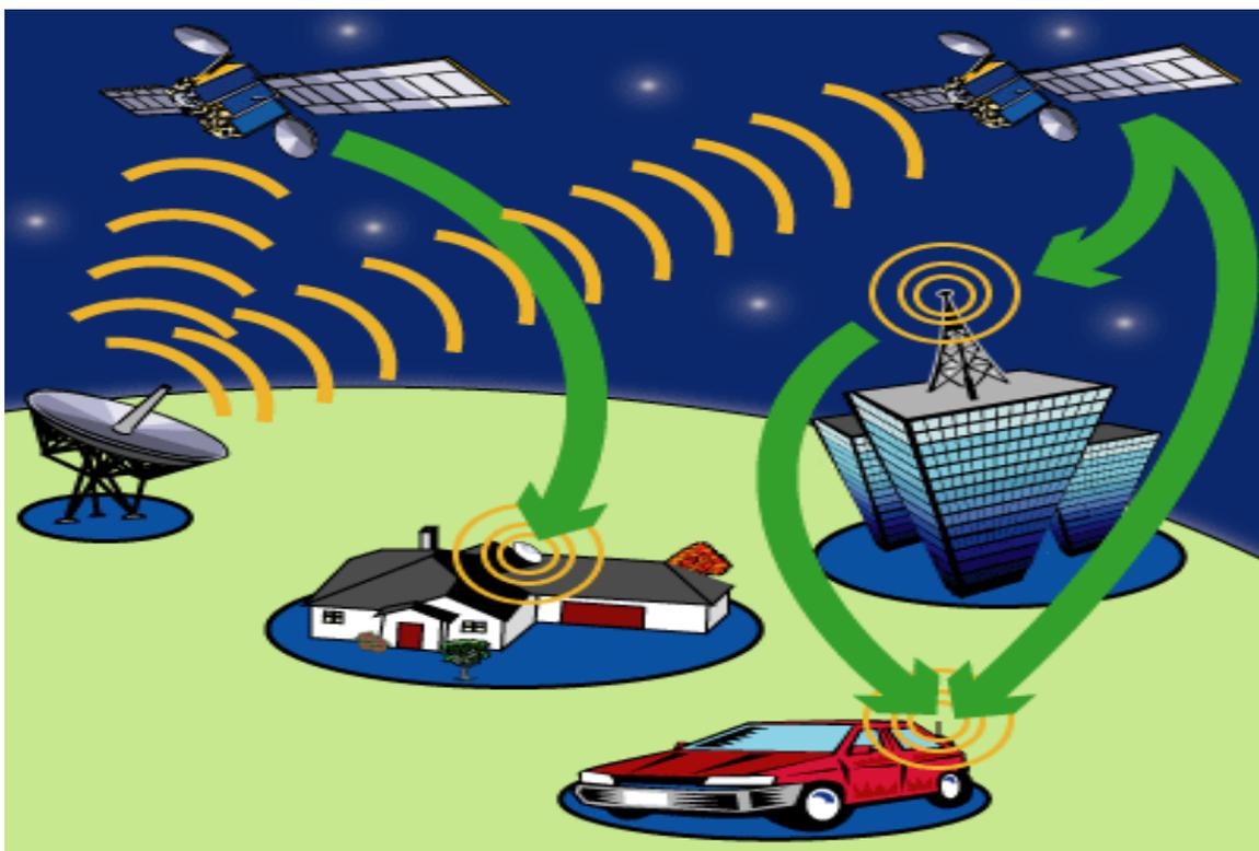
As the satellites orbit the earth, programs are beamed to them from broadcast stations. The satellites then transmit the signal to special antennas on homes, cars and portable radios. Terrestrial repeaters throughout the country also receive the signal and help ensure that it's transmitted to receivers, especially in areas with tall buildings that might block the signal
