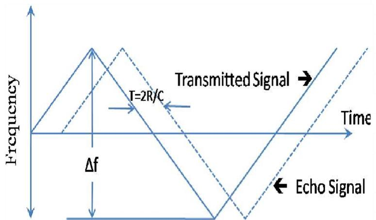
[ SAW TOOTH WAVE FORM IN FMCW RADAR ]
