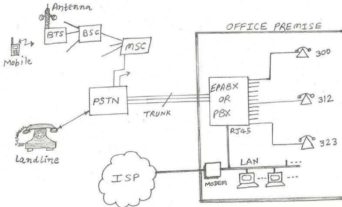
EPABX/PBX is connected to PSTN (Public switched Telephone network) via trunk lines; hence all can use one external voice line in time shared basis.
