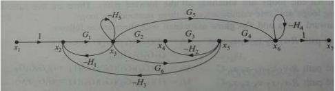
Q.10 Using mason gain formula find the transfer function  $\frac{c}{R}$  for the signal flow graph shown in figure.
