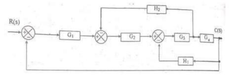
**Q.8** Find the overall transfer function of the system whose signal flow graph is shown below.
