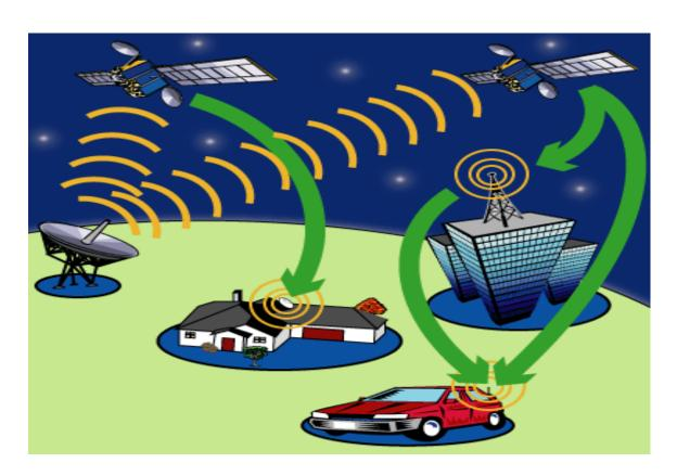
As the satellites orbit the earth, programs are beamed to them from broadcast stations. The satellites then transmit the signalto specialantennas onhomes, cars and portable radios. Terrestrialrepeatersthroughout the country also receive the signal andhelp ensure that it's transmitted to receivers, especially inareas with tall buildings that might block the signal
