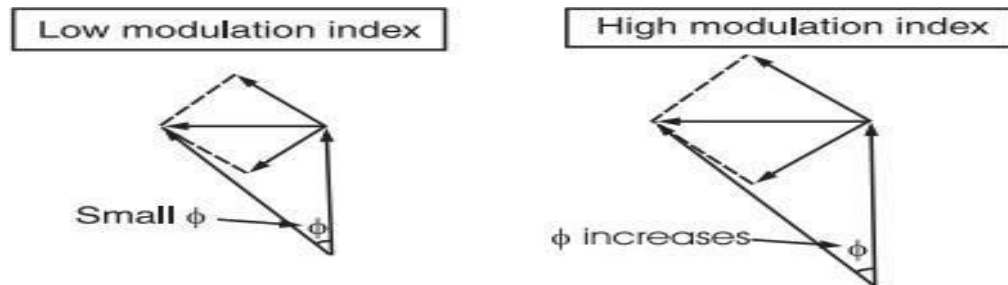
Fig.3 : Effect of modulation index on frequency f
