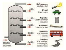
fractional condensation occurs at different heights of the distillation unit. Different fractions are collected from their respective outlets. The fraction with highest boiling point is collected at the bottom, while that with lowest boiling point is collected at the top.
