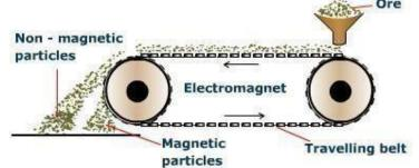
method a belt is tied over two rollers of which one is made up of magnet. Pulverized ore is added over the belt through a hopper. The pulverized ore move towards the magnetic pulley along with the rotating belt. The non-magnetic impurities fall directly below the magnetic pulley while the magnetic ore form a separate heap due to the influence of the magnetic field.
